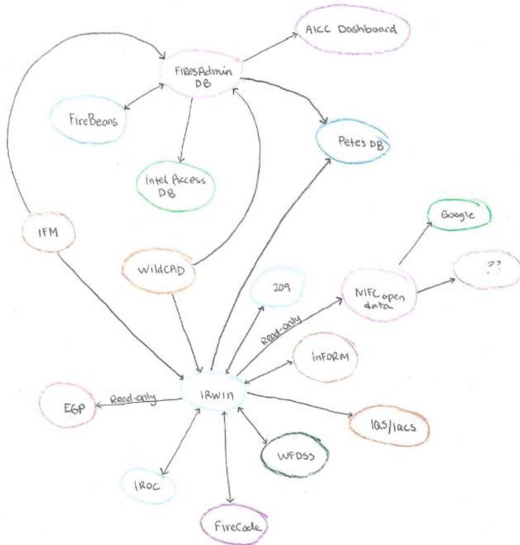
Figure 1 is a depiction of how the fire applications 'talk' to each other through IRWIN.
